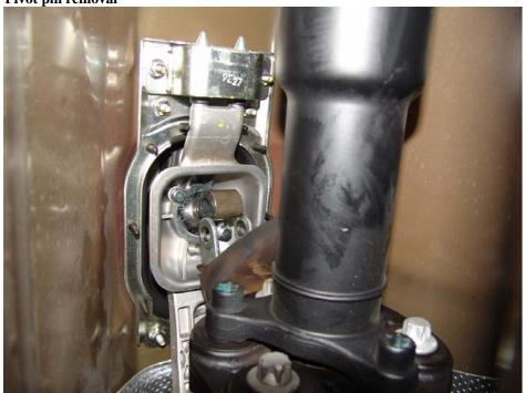
Figure 8: Shifter bolt removal
