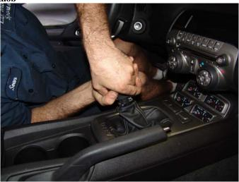
Once the shift knob has been removed you can now remove the lower shifter trim plate from the car. Again this piece is held in with small GM clips. You may find it easier to use a small flat blade screw driver, or clip removal tool. See figures 2a and 2b.
