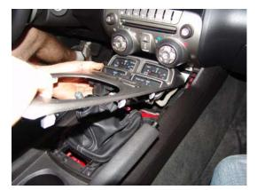
With the trim panel up, becareful of the gage package wiring. There should be enough wiring there to allow this panel to be laid over to the side out of the way. Next you will be removing the lower shift boot from the transmission tunnel. These are held down with four Philips head screws. See figures 3a and 3b.
